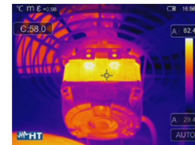
3 rd photo: thermogram of an electric motor acquired with THT300.
