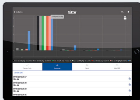
Current and voltage harmonics.
