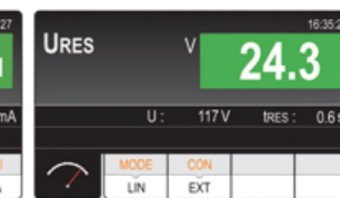
Residual voltage measurement.
