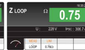
Measurement of Loop impedance.
