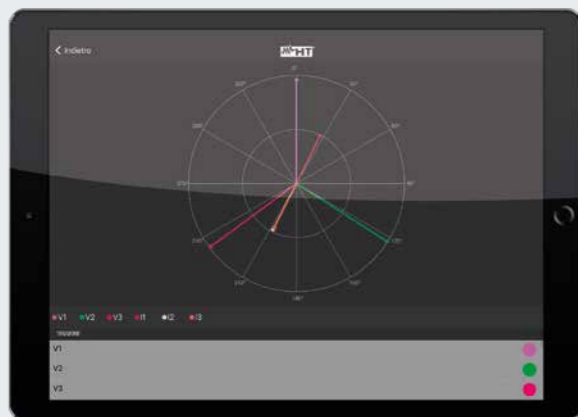
Voltage and current vector diagram.
