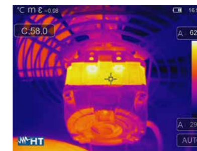
3 rd photo: thermogram of an electric motor acquired with THT300.
