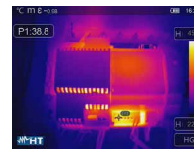
2 nd photo: thermogram of a power supply acquired with THT300.
