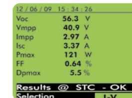
Detail of the single results of Curve I-V: OK
