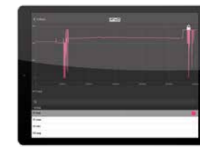
Example of display Recording made (evident voltage interruptions)
