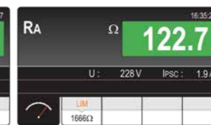
Measurement of overall earth resistance.
