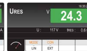
Residual voltage measurement.
