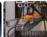
Measurement of leakage current with optional clamp HT96U.
