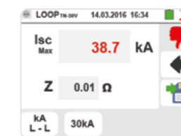
Advanced Loop: negative result of interruption power test.
