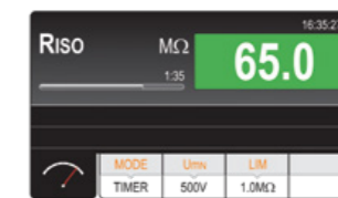
Measurement of insulation resistance.
