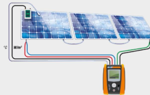
MISURA DELLA CURVA I-V CON SENSORI CONNESSI DIRETTAMENTE AD I-V500w
