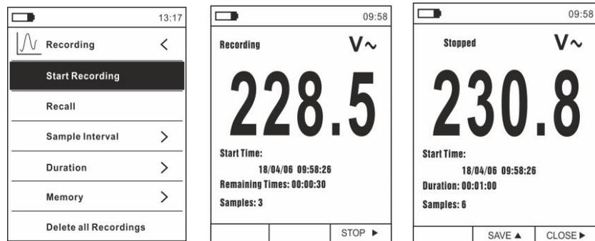
**Fig. 37:** Data logger function – Starting and stopping recording
