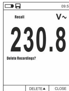
**Fig. 40:** Data logger function – Deleting recorded data
