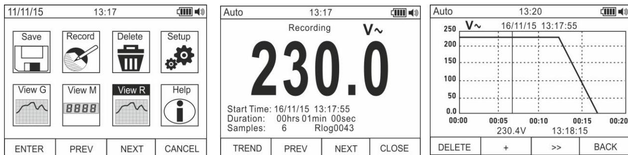
Fig. 20: Recalling recordings to the display
